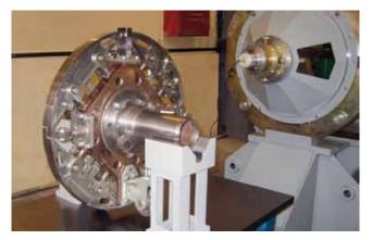
Additional machining devices for torpedo tube guide tracks upon onboard installation at construction, repair and modernization stages to ensure torpedo projection.
